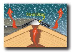
material, Trimline vents fit a variety of roof styles including shingle, cedar, tile and metal. Designed to vent at the ridge the hottest point of the roof – the Trimline vent system has the added benefit of creating a smooth roofline, eliminating the unsightly louver vents commonly found on
